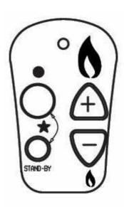
To adjust to the minimum setting press the lower right hand triangular button indicated by the small flame and the minus symbol until the audible beep is heard, immediately let go of the button. The fire will then go to the minimum setting.
